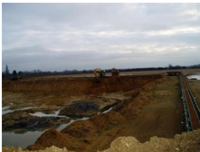
Picture 2 Extracting glacial sand and gravel at Broom quarry.
